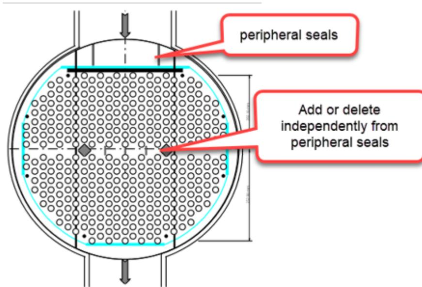
The effect of any changes to sealing strips or other means to block pass lanes will be reflected in the cross flow fractions and thus in the heat transfer calculations.
