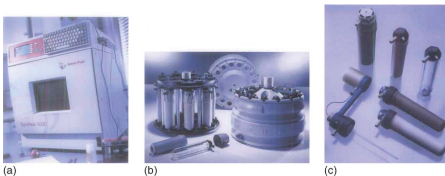
Figure 16 (a) The Anton Paar Synthos 3000 with (b) rotors and (c) vessel types. (Courtesy of Anton Paar GmbH.)
