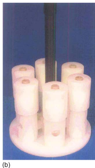
Figure 12 (a) The Milestone MonoPREP module and (b) its parallel setup rotor PRO-6 (right). (Courtesy of Milestone s.r.l.)
