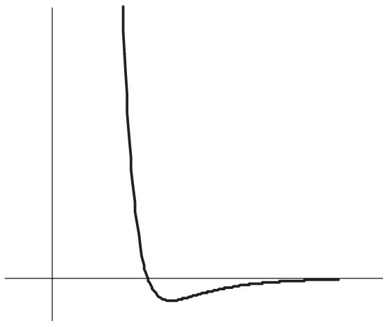
Figure 5 Schematic illustration of the Lennard-Jones potential, showing the steep repulsion as atoms approach each other, the minimum, and the asymptotic approach to zero potential energy as the atoms move further apart.
