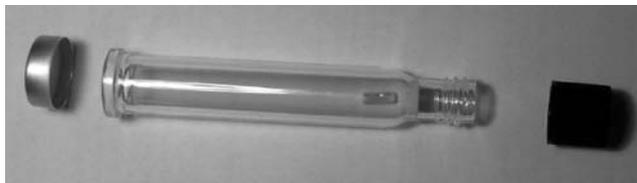
**Fig. 8** Modified Smith process vial for microwave-assisted solid-phase organic synthesis
