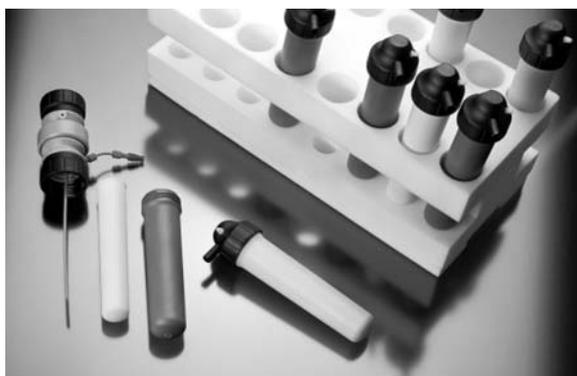
**Fig. 9** The SPOS-compatible reaction vessel for the Synthos 3000. Depicted from *left to right* is the filtration unit, the PTFE liner (*white*), the pressure jacket, and a fully assembled vessel with a ceramic pressure jacket
