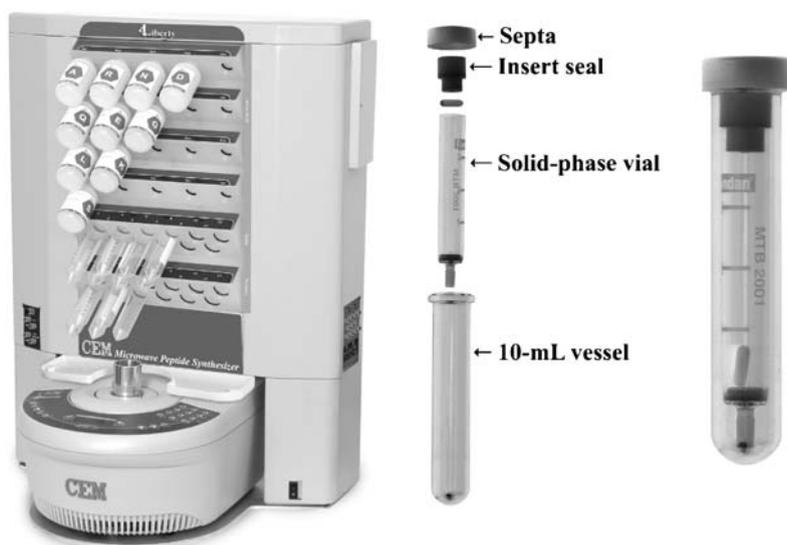
**Fig. 10** Liberty (CEM Corporation), the first automated microwave solid-phase peptide synthesizer, is shown on the *left*; the available reaction vessel setup for solid-phase synthesis is depicted on the *right*
