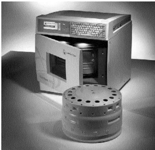
**Fig. 2** Synthos 3000 bench-top multimode microwave apparatus of Anton Paar
