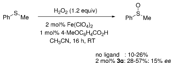
Scheme 18.2 Iron-catalyzed oxidation of phenylmethylsulfide with hydrogen peroxide in the presence and in absence of 3g .
