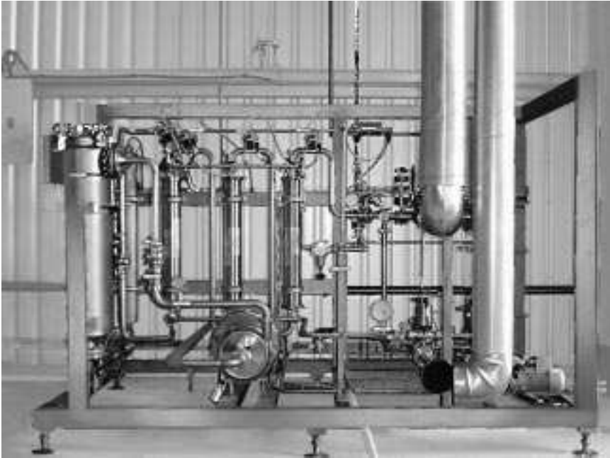
Fig. 9.14 Erox deaeration plant (Source: EUWA).
