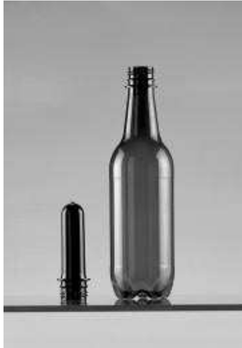
Fig. 14.1 Shows a preform and a stretch blow moulded bottle. Courtesy Kronos UK.
