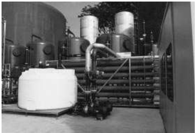
Fig. 9.10 Reverse osmosis plant (Source: EUWA).
