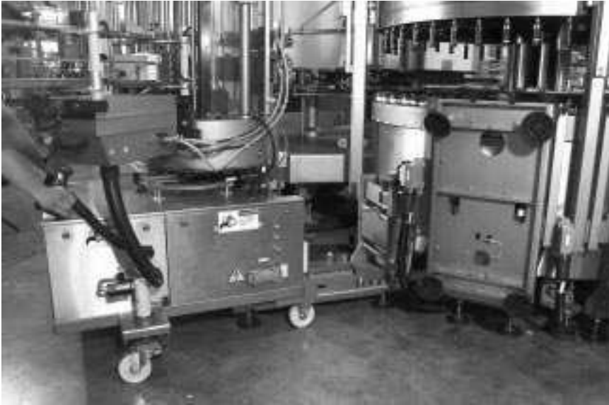
Fig. 14.3 Shows an interchangeable labelling station on a wet glue/PSL labeller. Courtesy Kronen UK.
